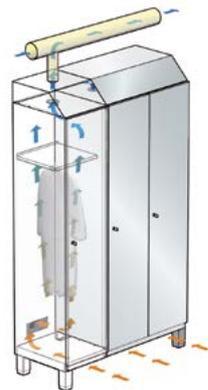
Our FVL technology means a high air renewal rate thanks to connection to the customer's ventilation system.
