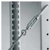
Diagonal brace with tightener
